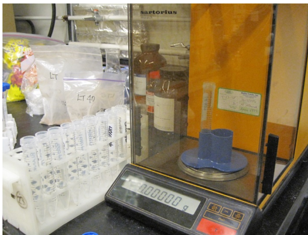
Figure 22 Analytical balance and 15 mL centrifuge tube with tube base.
