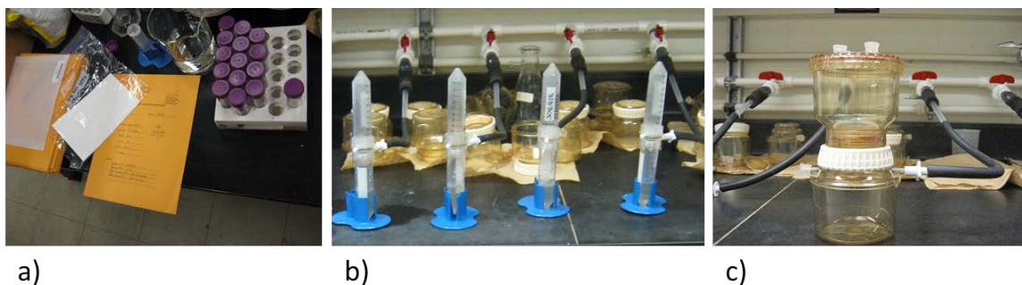
Figure 19 PM 10 aerosol extraction process. a) PM 10 filter removal into aerosol solution, b) steriflip filter system, and c) vacuum filtration system.
